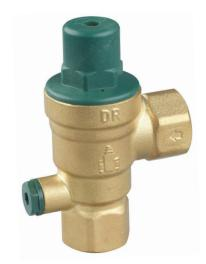
Pressure Reduction Valves are fitted in water systems to moderate and stabilise mains water pressure, which is at times too high for domestic appliances. The valves are pre-set at 500kPa which is the most widely used setting for domestic appliances. However the pressure reduction valves can be easily adjusted to suit your needs from a range of 150kPa to 600kPa.
